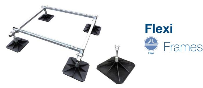
The BASE & EXTENDER frames are designed to provide stability and spread loads evenly across flat roof surfaces. The galvanised steel frame raises equipment up to 405mm above the flat roof level, permitting quick and easy access for roof maintenance.
